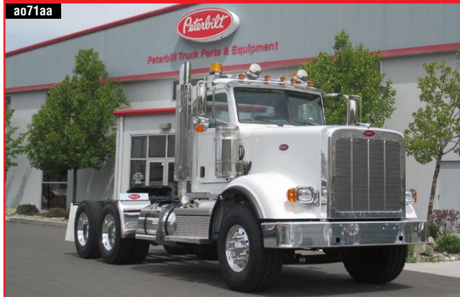
2018 PETERBILT 367 Cummins X15, 565 HP, 18 Spd, Air Trac Susp, 205" WB, 22 FA, 46 RA, 10-3/4x 3/8's Frame With Full Liner, Lockers.
